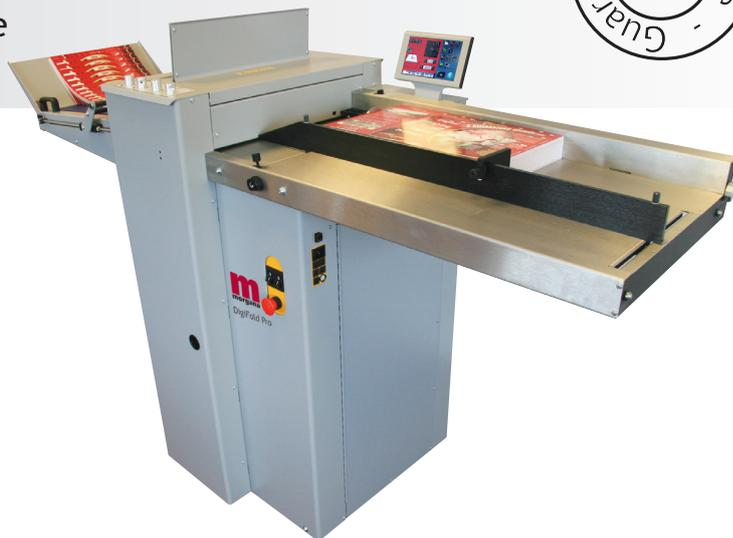
repeatable quality of the DigiFold Pro. The maximum sheet size is 700mm x 385mm (900mm x 385mm with optional extension table) allowing a wider range of jobs to be tackled. Perforation is also standard on the DigiFold Pro with up to 5 perforation wheels being used across the sheet.
