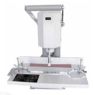
VS-55 is the standard model tabletop drill. By rotating the pre-programmed pitch bar dial, the desirable hole pitch can be selected from several pitch patterns.
