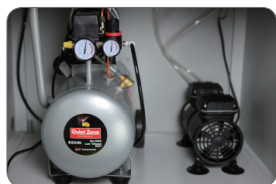
Air Compressor / Vacuum Pump
